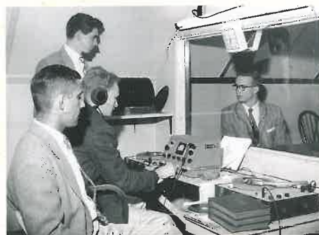
Top left, the early days of radio at Nichols Junior College. Top right, the 1958 studio boasted a "control room with a 50-watt transmitter, two three-speed turn tables, a two-speed tape recorder, record recorder, two dynamic microphones, one Cardyne microphone, Slim Trim microphone, floor stands, boom, and two monitors."
